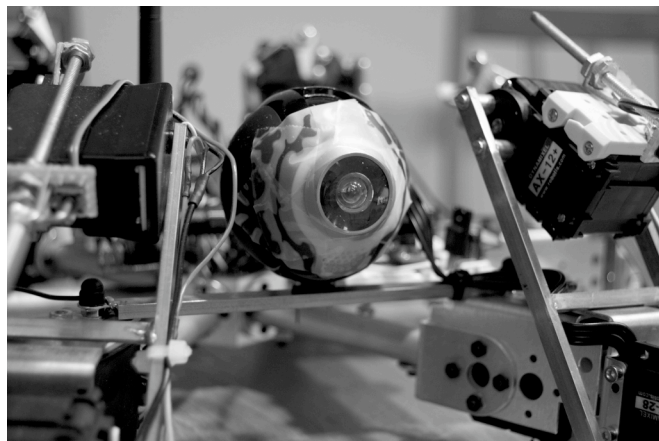
Fig. 2. Quickcam Communicate Deluxe web cam used for vision. A door peephole was disassembled and quickly mounted to greatly improve the field of view, resulting in better orientation measurements from optical flow.
